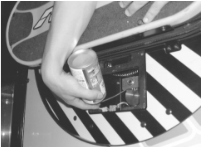
PHOTO 10. 3 k YAW-Direction Volume Control Mechanism Assembly
