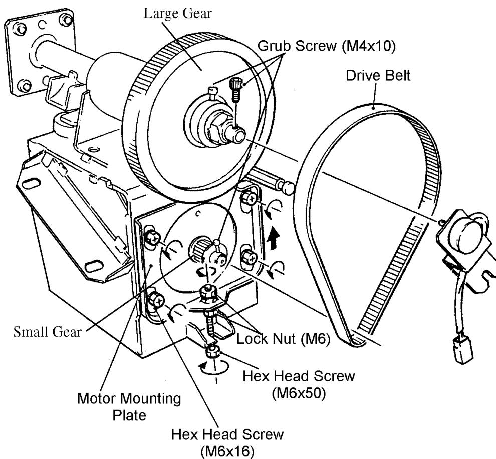
4. Slacken the Lock Nuts (M6) and Adjustment Screw (M6x50), to remove the tension from the Drive Belt, and remove the Drive Belt.
