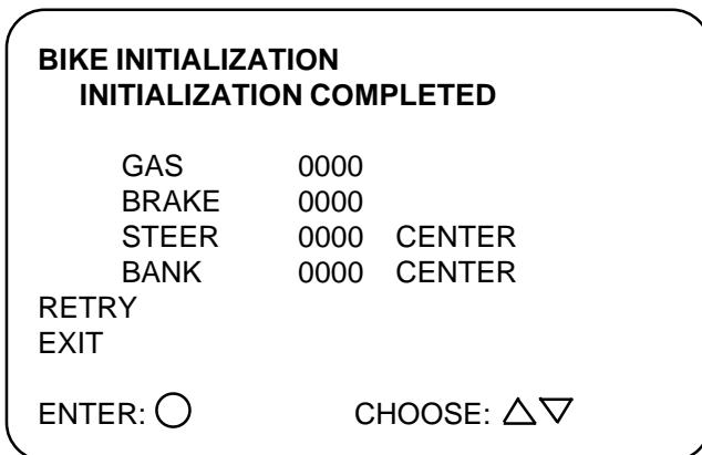
4. When the value of ‘GAS’, ‘BRAKE’, ‘STEER’, and ‘BANK’ is around ‘0000’, and ‘OK’ is displayed when each item is operated, the adjustment is completed. Otherwise, select ‘RETRY’ to readjust the unit.
