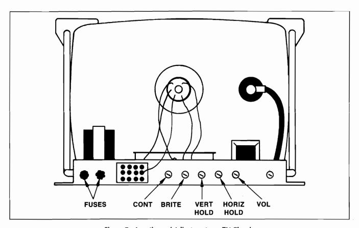
Figure 7 Locations of Adjustments on TV Chassis
