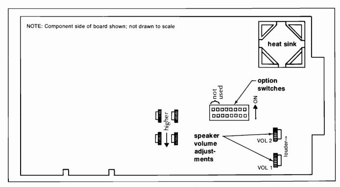
Figure 2 Approximate Locations of Option Switches and Sound Pitch, Tachometer and Volume Pots
