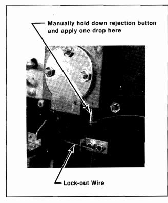
Figure 14 Close-up View of Lubrication Point
