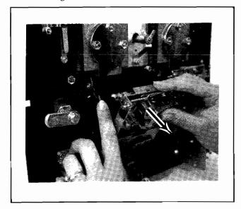
Figure 11 Removal of Coin Mechanism
