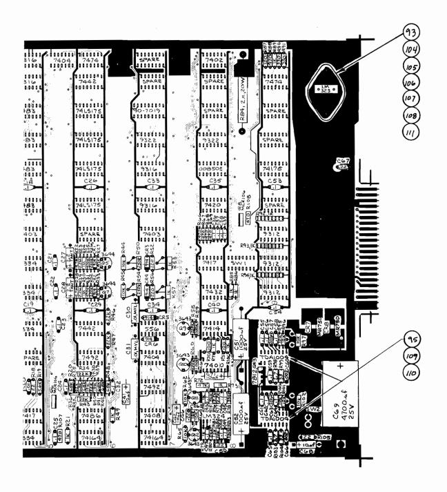
Figure 21 Game PCB Assembly Drawing and Parts List
