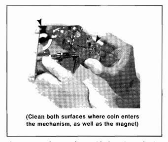
Figure 12 Surfaces to Clean Inside the Coin Mechanism
