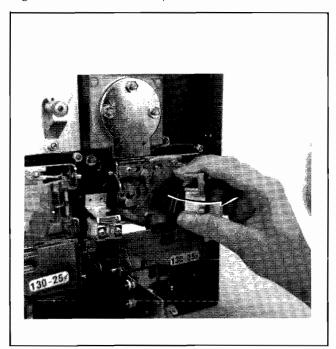
Figure 10 Hinging Open the Magnet Gate Assembly
