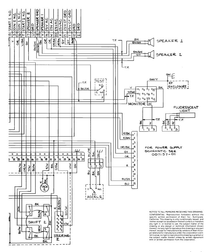
Figure 22 Harness Schematic
