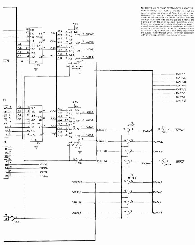
Figure 20 Game PCB Schematic Diagram Sheet 4 of 7
