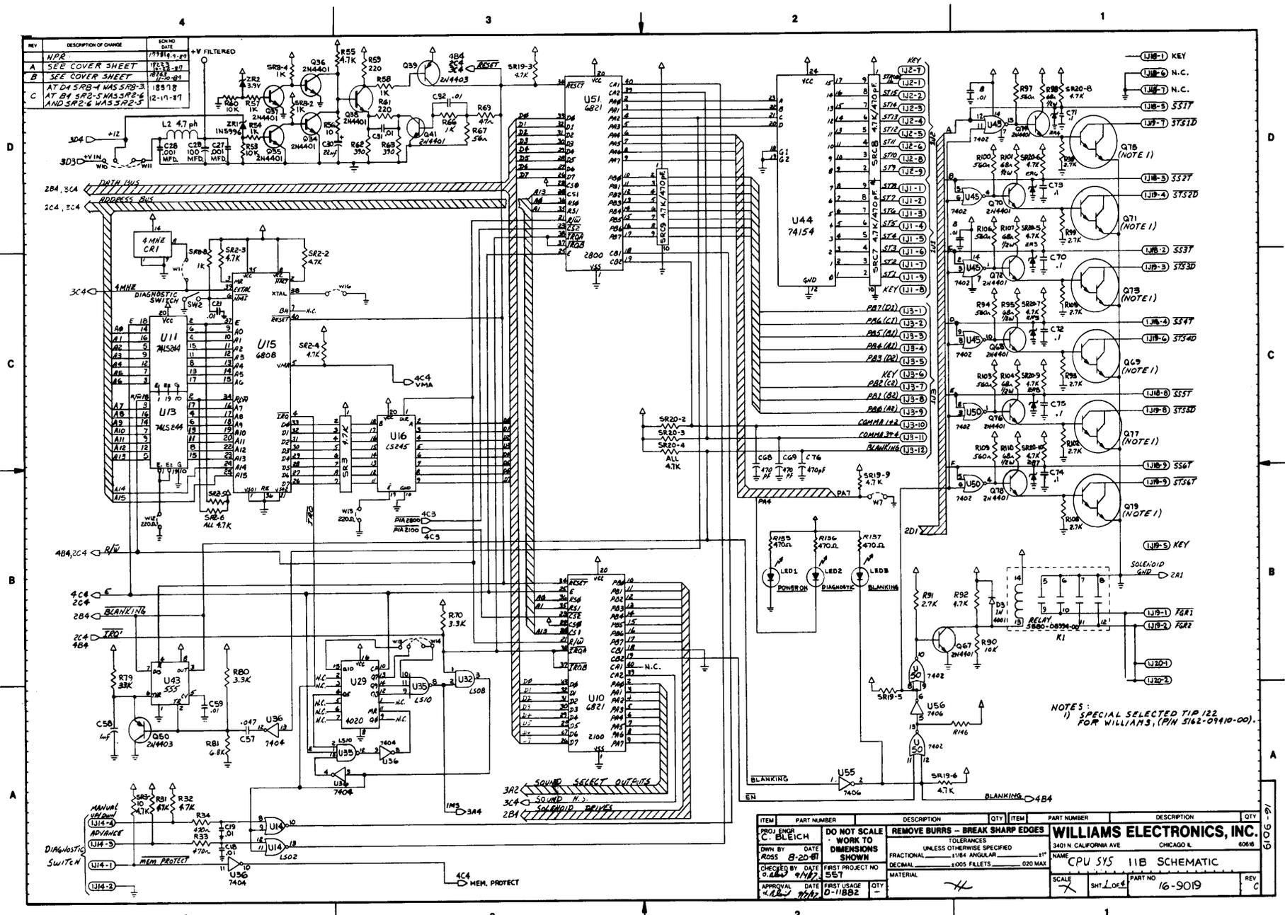
System 11B CPU Schematic (16-9019, Sheet 1 of 4)
