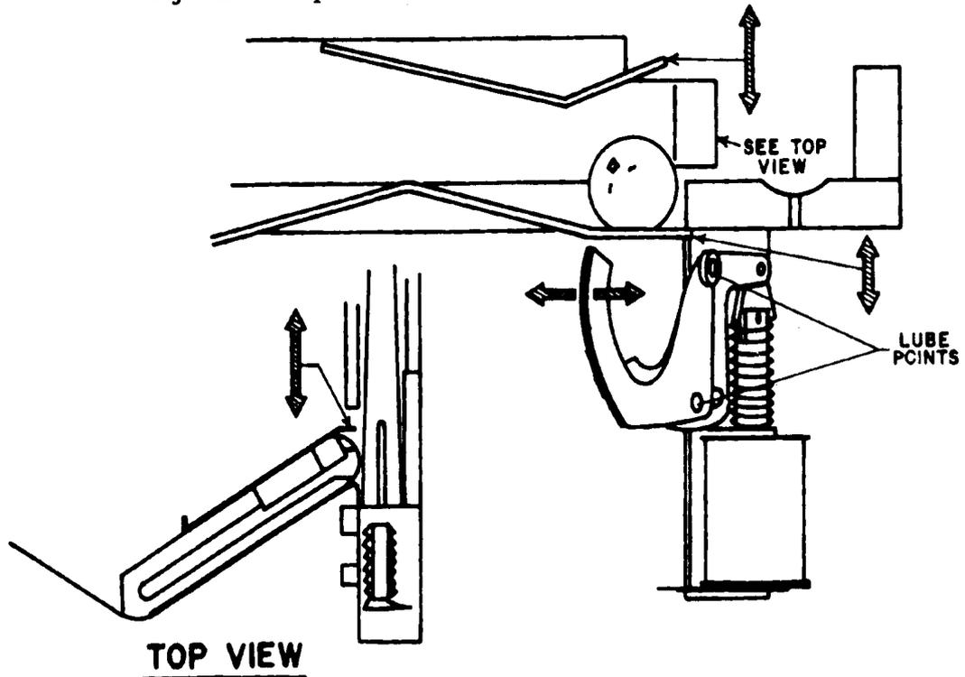
Figure 5. Adjustments and Lubrication Points, Shooter Lane Feeder
