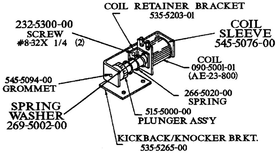
KICKBACK ASSEMBLY 500-5080-00 (COIL LUGS ON THE SIDE )
