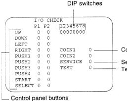
The various switches on the control panel and elsewhere can be checked.
