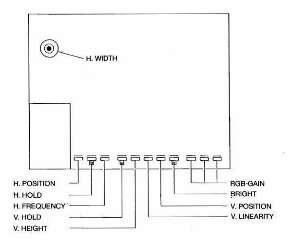
The adjustments have been done at the factory for the best performance, but if necessary, adjust the above pots by referring the explanation for each adjustment.
