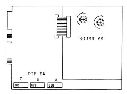
o SOUND VR  $\cdots$  Potentiometers for adjusting the sound volume.
