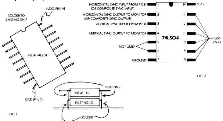
CURE 2: Used for Wells-Gardner Video-Sync boards with positive sync connections only. (Vertical mount board 85x140B.
