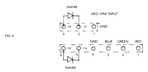
CURE 3: Join negative sync inputs J2 and J3 together with a jumper. Locate W102 and install a jumper from W102 to either J2 or J3.
